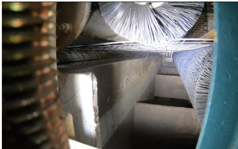
The interior of the dual brush roll system, with wire mesh moving between the brushes
